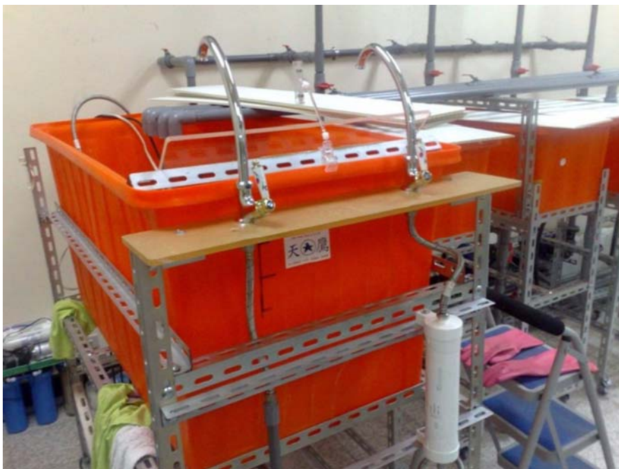
Figure 3. Close up of the system - A model plumbing system with two goose neck faucets and a Nephros filter.
