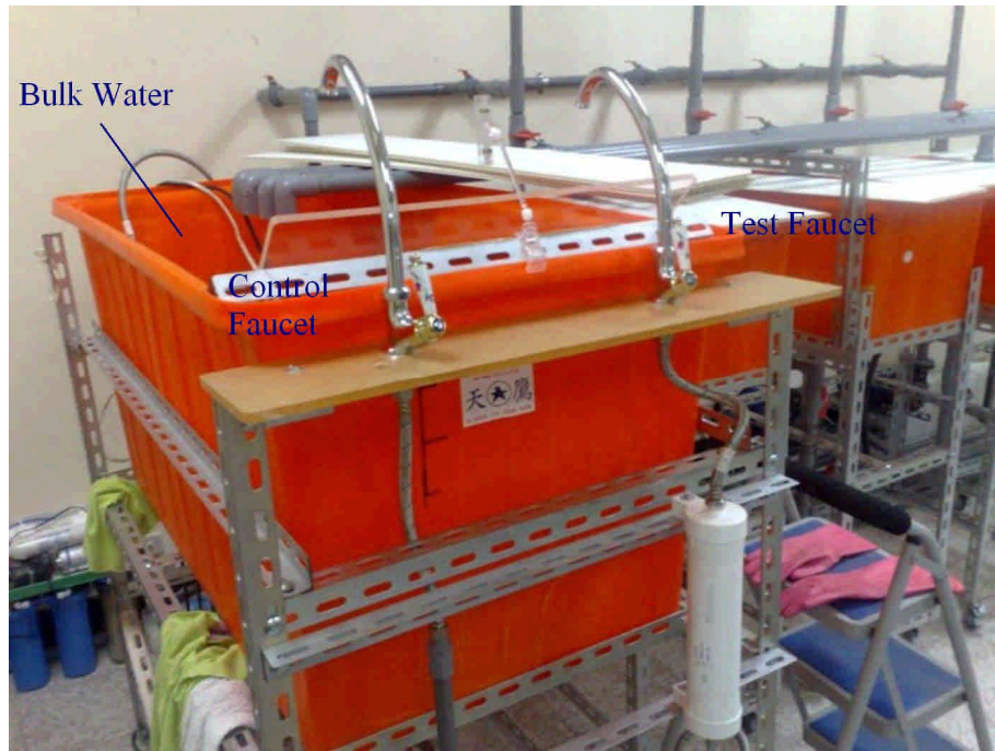
Figure 2. A model plumbing system with two goose neck faucets and a Nephros filter.
