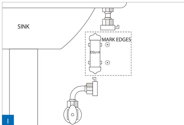
1. PLACE filter vertically against wall in a position that both flex lines are not stretched.
