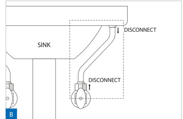
1. DISCONNECT, REMOVE, and DISCARD the current flex lines on both sides of sink.
