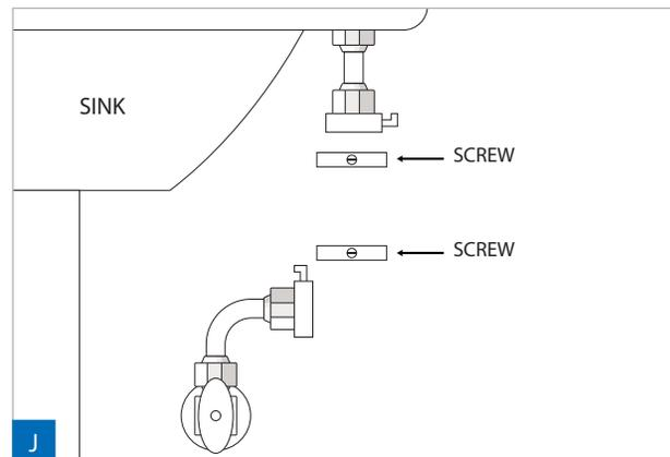
1. MOUNT the c-clamps with 2 screws (1 each).
