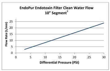
1. Maximum Flow Rate per 10" Segment = 2.5 GPM
