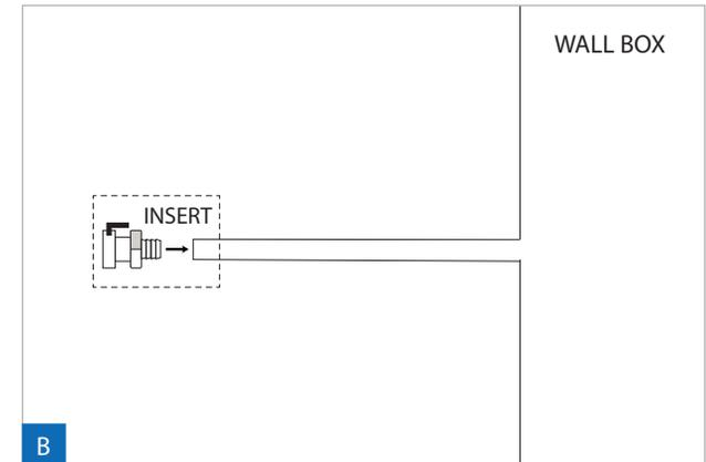
1. INSERT a quick connector to the free end of the old hose previously disconnected from the dialysis machine.
