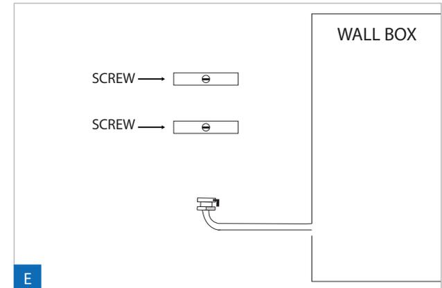
1. DRILL holes at the marked locations for the screws and MOUNT the clips with their enclosed screws.
