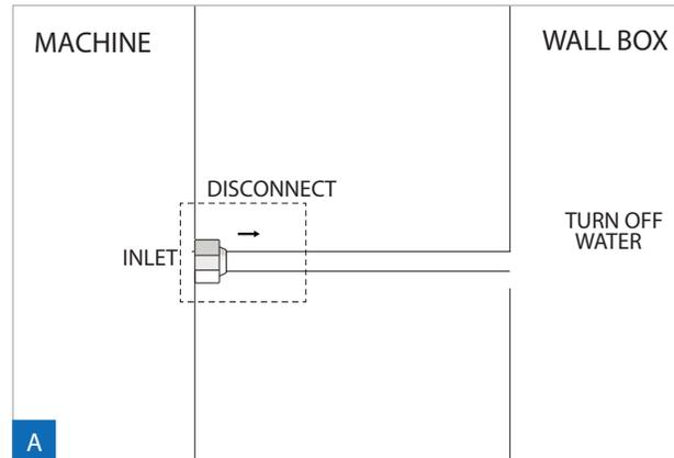
1. TURN OFF the water supply to the dialysis machine from wall box or RO outlet.
