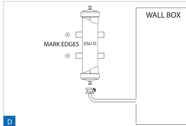
1. PLACE the filter vertically against wall near wall box or on frame of individual RO cart in the position it will be mounted.
