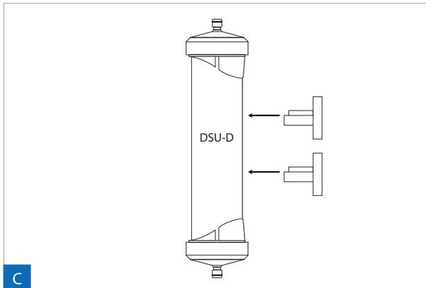
1. PRESS both clips (one clip for SSU) into the DSU filter.
