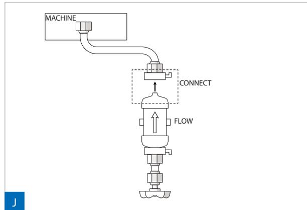
1. CLIP the filter to the c-clamp so the flow symbol on filter is toward the machine's inlet.
