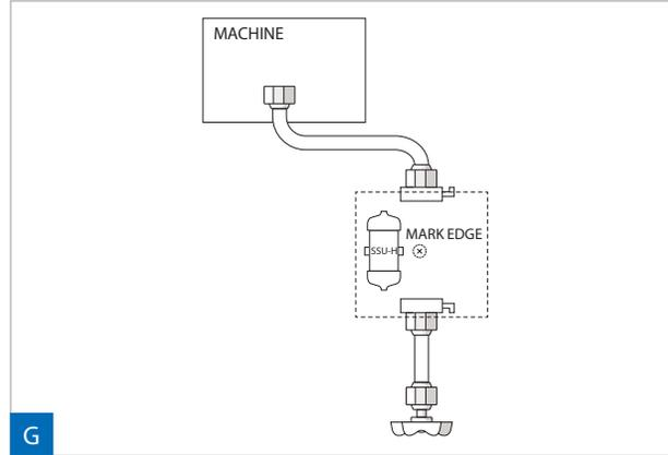
1. PLACE filter vertically against a surface near the machine in a position that both flex lines are not stretched.
