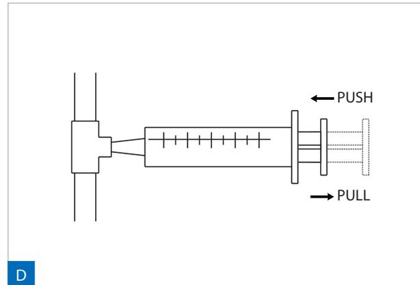
1. PULL out syringe plunger to draw the germicidal disinfectant.
