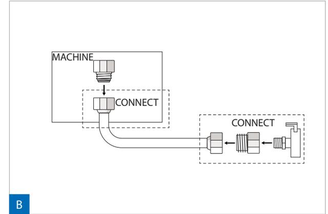
1. CONNECT a new flex line to the machine's inlet.
