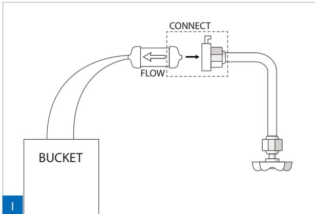
1. CONNECT the filter to the quick connector of the water valve so the FLOW direction is towards the flow of water.
