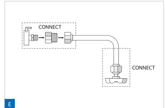
1. CONNECT a new flex line to the water valve.
