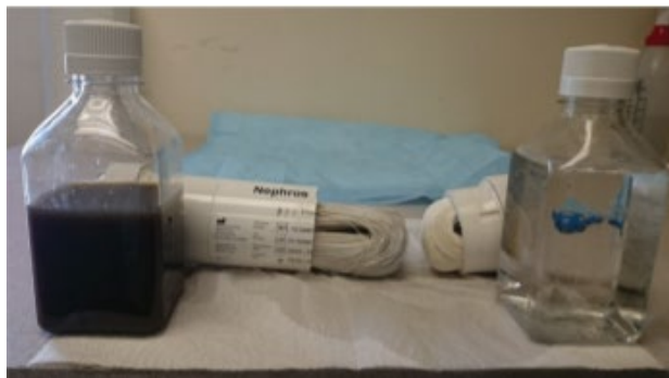
Typical removal results of a Nephros filter
