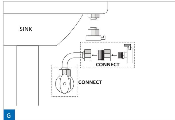
1. CONNECT the water valve flex line to the water valve by the 3/8" compression fitting.
