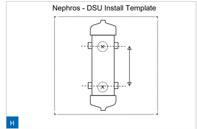
1. ATTACH the DSU template (provided in installation kit) vertically against the wall in a desired position to ensure that both flex lines are not stretched.
