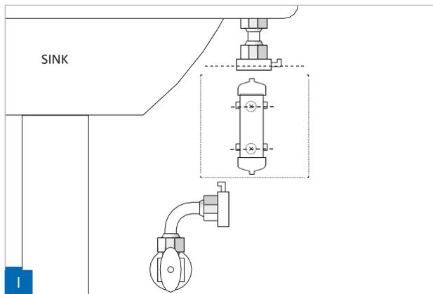
1. MARK the hole locations of the c-clips on the wall.
