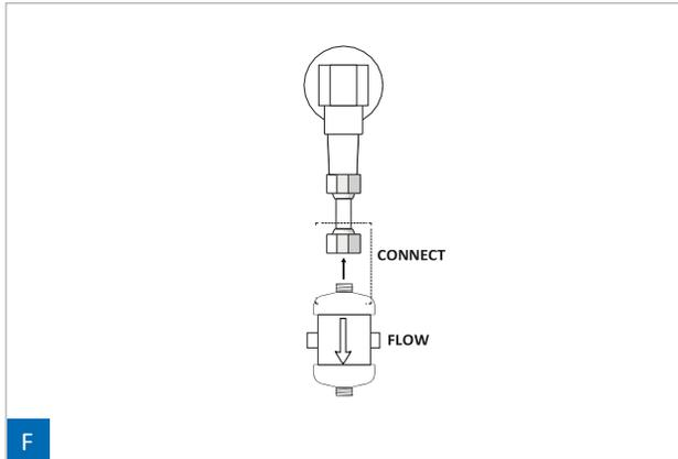
1. CLIP the filter so the FLOW direction is towards the flow of water, pointing away from the water supply pipe.
