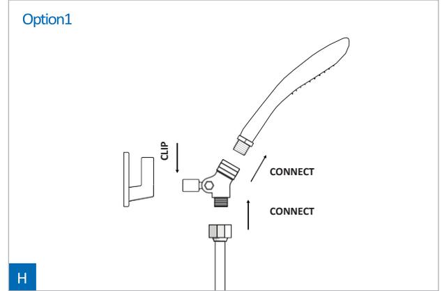
1. CONNECT the female connector on the shower hose to the Swivel Connector.
