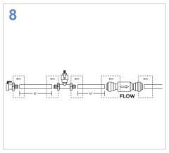
CONNECT quick connector to a new tubing line.
