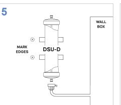
PLACE the filter vertically against wall near wall box or on frame of individual RO cart in the position it will be mounted.
