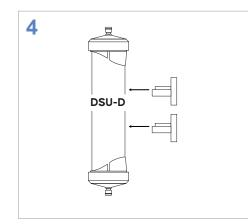
PRESS both clips (one clip for SSU) into the DSU filter.
