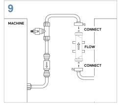
CONNECT the water line from wall box or RO outlet with the quick connector to the filter's inlet.
