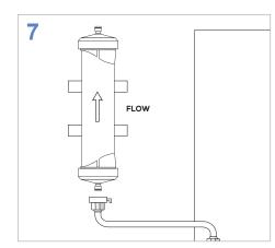
PRESS the filter into the clips so that the direction of flow is towards the water flow, which is towards the dialysis machine.
