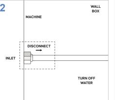
TURN OFF the water supply to the dialysis machine from wall box or RO outlet.
