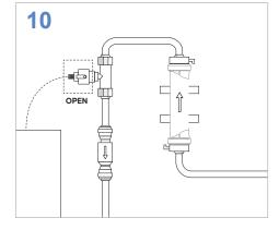
PLACE a bucket under the sample port to catch the water that will be exiting.
