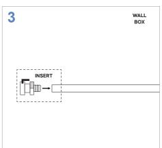
INSERT a quick connector to the free end of the old hose previously disconnected from the dialysis machine.
