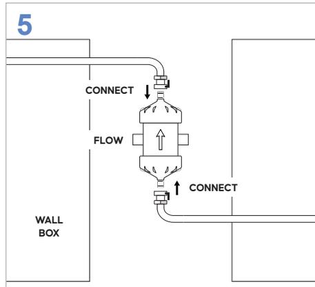
PRESS the filter into the c-clip so the direction of flow is towards wall box.
