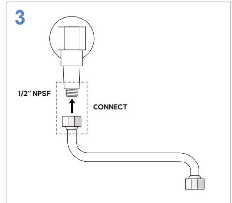
**3** CONNECT a new flex line by the 1/2" NPSF fitting to the water supply pipe.
