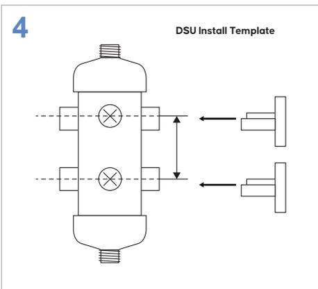
**4** ATTACH the DSU Template (provided in installation kit) vertically against the wall in a desired position to ensure that both flex lines are not stretched.
