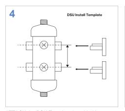
ATTACH the DSU Template (provided in installation kit) vertically against the wall in a desired position to ensure that both flex lines are not stretched.
