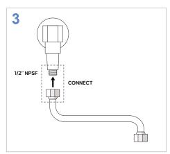
CONNECT a new flex line by the 1/2" NPSF fitting to the water supply pipe.
