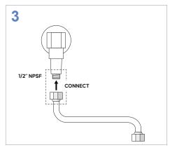
CONNECT a new flex line by the 1/2" NPSF fitting to the water supply pipe.
