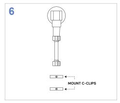
MOUNT the C-Clips with 2 screws (1 each).
