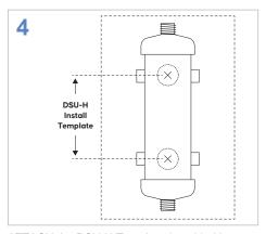
ATTACH the DSU-H Template (provided in installation kit) vertically against the wall in a desired position to ensure that both flex lines are not stretched.
