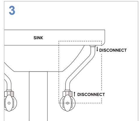
DISCONNECT, REMOVE, and DISCARD the current flex lines on both sides of sink.
