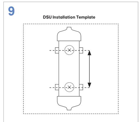
ATTACH the DSU template (provided in installation kit) vertically against the wall in a desired position to ensure that both flex lines are not stretched.
