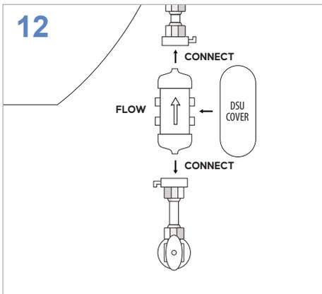
REMOVE blister pack and CLIP filter to the C-Clips so the flow symbol on filter is towards the faucet.
