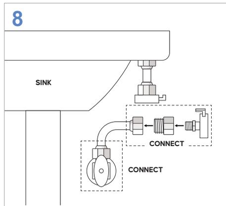
CONNECT the water valve flex line to the water valve by the 3/8" compression fitting.
