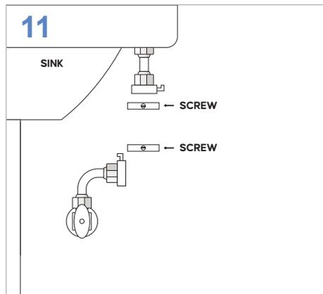
MOUNT the C-Clips with 2 screws (1 each).
