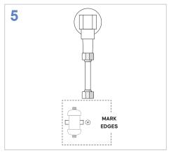
PLACE filter vertically against a surface near the water supply pipe in a position that the flex line
