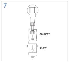
CLIP the filter so the FLOW direction is towards the flow of water, pointing away from the water supply pipe.
