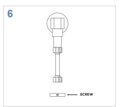
MOUNT the c-clamp with one screw, lining up the edge of the c-clamp with the mark previously
