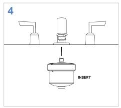
INSERT the S100 Point of Use filter into the aerator adapter.
