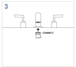
If an aerator adapter needs to be installed, CONNECT the aerator adapter into the faucet opening. The aerator adapter thread size should match the faucet thread (e.g. 55/64" or15/16").
