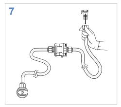
THREAD the QC assembly that was set aside into the other end of the new flex line.
