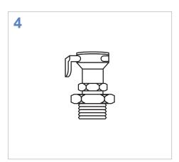
UNSCREW the QC assembly from the water valve flex line (do not disassemble the QC assembly) and set aside.
