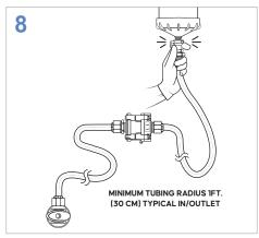
CONNECT the new flex line's QC assembly to the inlet of the DSU filter.
