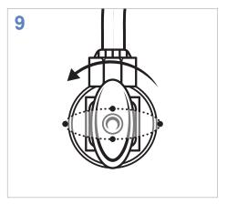
Turn ON water supply valve and check for leaks.
