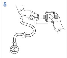
THREAD the water valve flex line's 1/2" NPSF fitting to the inlet side of the PRV (identify that arrows on PRV follow flow direction).
