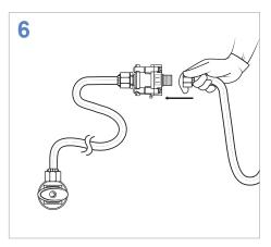
THREAD the new flex line to the outlet side of the PRV.
