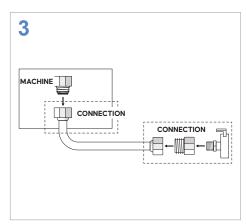
CONNECT a new flex line to the machine's inlet.
