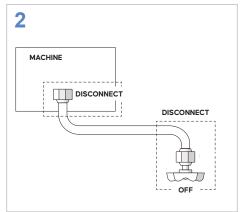
TURN OFF the water supply valve. DISCONNECT the supply line from the machine's inlet and water valve.
