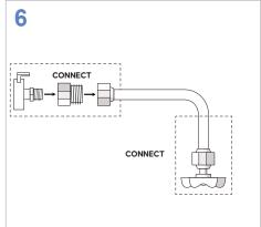
CONNECT a new flex line to the water valve.
