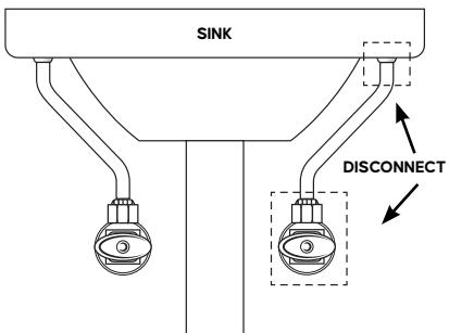
DISCONNECT, REMOVE, and DISCARD the current flex lines on both sides of sink.
