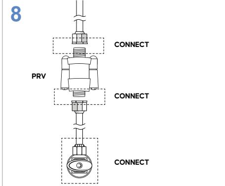
CONNECT the water valve flex line to the water valve 3/8" compression fitting.
