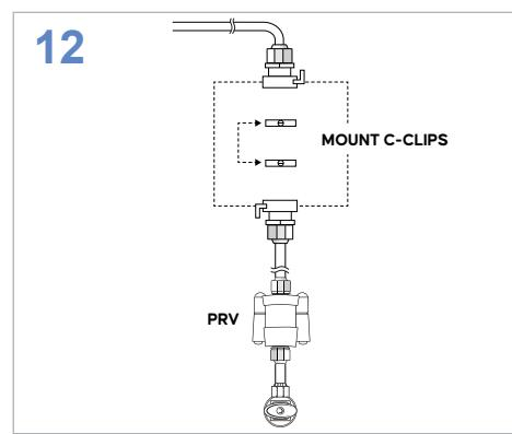
MOUNT the C-Clips with 2 screws (1 each). DO NOT REMOVE the blister pack. PUT ON new gloves.
