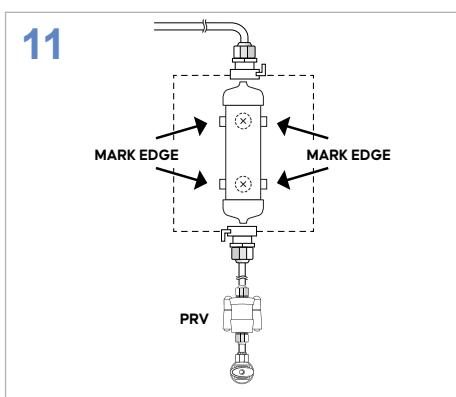
MARK the hole locations of the C-Clips on the wall.
