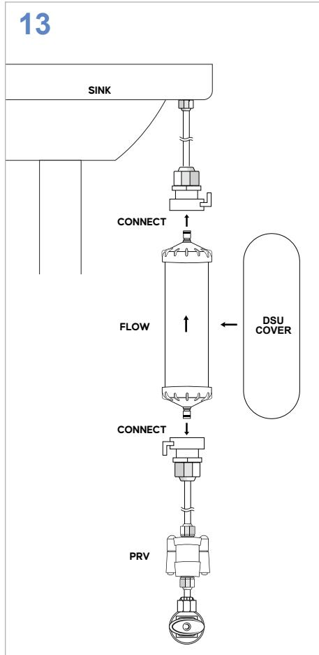
REMOVE blister pack and CLIP filter to the C-Clips so the flow symbol on filter is towards the faucet.
