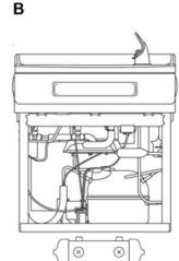
NOTE: Side **A** in graphic shows dual unit with space for filter inside the unit; Side **B** in graphic shows a single unit with filter placed outside the unit.
