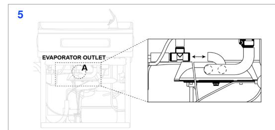
DISCONNECT outlet (brass) tubing of evaporator from tee/union going to bottle filler / fountain dispenser at location (A). This tubing may be 1/4" or 3/8".
