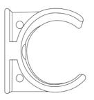
INSTALL C-Clips with provided self-tapping screws (Reference Install Kit - Bottle Filler / Fountain, 70-0346) or adhesives (reference Drill Free C-Clip Anchor Kit, 70-0345) as defined by DSU template.
