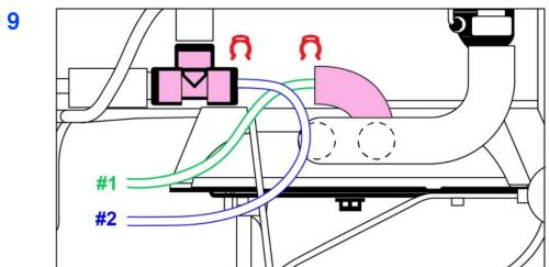
CONNECT end of tubing #1 to evaporator. Push-fit end of tubing #2 to tee/union.
