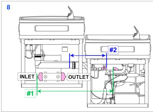
CUT new 3/8" tubing to be used before and after the DSU-H. Be sure to account for an adequate bend radius (≥ 1.25") when determining lengths of each piece of tubing.
